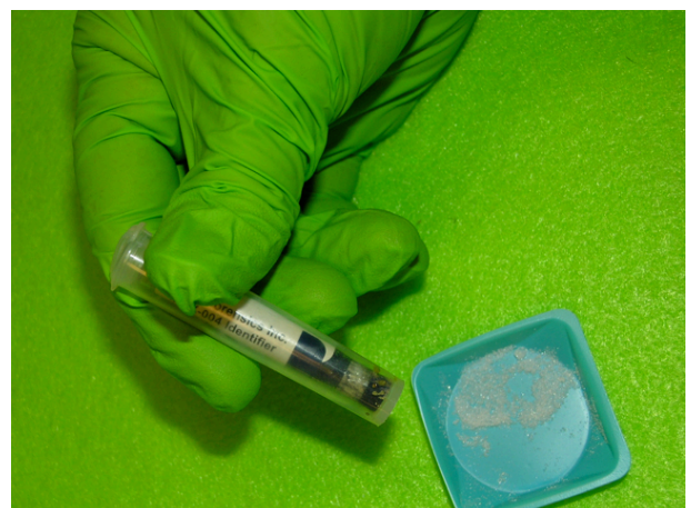
Example of chlorate positive (IDEX-004) - sampler tip turns from white to dark blue.
