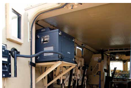
Vehicle mount with integrated real-time vapor sampling
